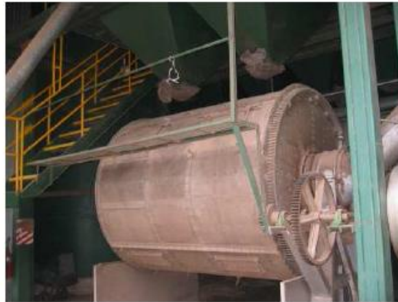
Figure 6: Coffee drying, Coopeldos, Costa Rica; (capacity 595 \text{ kW}_{\text{th}} , collector area: 850 \text{ m}^2 ) 6
